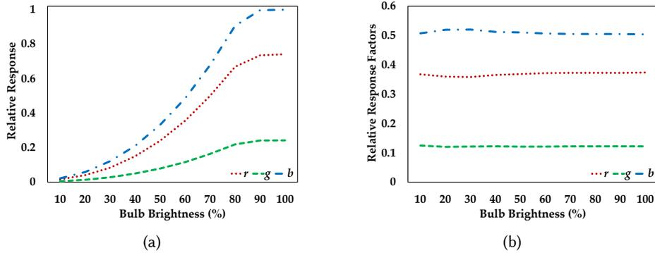
Fig. 6. (a) Observed response of  $\langle r, g, b \rangle$  components  $\langle \delta_r, \delta_g, \delta_b \rangle$  for  $RGB\langle 1 : 1 : 1 \rangle$ , and (b) Response factors for  $RGB\langle 1 : 1 : 1 \rangle$  at different brightness levels.
