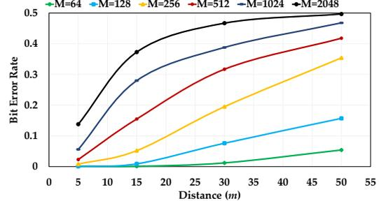
Fig. 16. Mean BER in exfiltration of both text and image.
