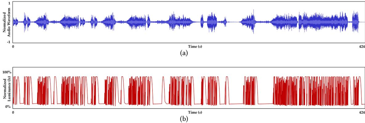
Fig. 3. (a) Audio waveform of *Beethoven's 5th Symphony* (duration of 7 minutes and 4 seconds); (b) Fluctuations in brightness of an audio-visualizing smart bulb output (in static hue mode), as captured by a BH1751FVI luminance meter.
