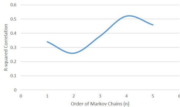
Figure 5.9: Reconstruction accuracy measured in terms of R-squared correlation when data was perturbed using a random sampling rate.
